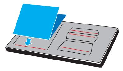
1. Use a folded piece of paper large enough to cover the large square on the die. Align the folded edge of the paper with the crease rule (red).
