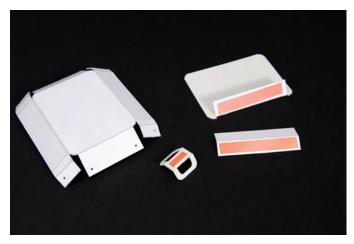
1. Die-cut material of choice, fold and apply adhesive as shown. The piece on the top right is the lid. The piece on the bottom right is the closure flap. The lid flap should be folded over all the way while the closure flap should be only lightly folded.
