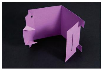
1. Die-cut from chosen material and fold as shown. Everything should be folded toward the center, including the pointed end flaps.
