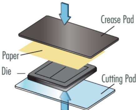
Place an Originals or Bigz Die on a Cutting Pad with foam side up. Place paper or desired material to be cut on top of the die. Place the second Cutting Pad or Premium Crease Pad on top of the paper or material to create a "sandwich."
