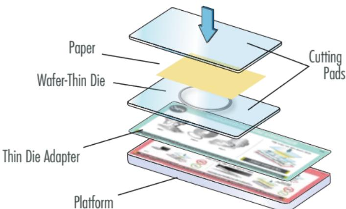
When using wafer-thin dies, a Thin Die Adapter is required and is placed directly on top of the platform. Create the "sandwich" by placing wafer-thin die onto Cutting Pad with blade side up. Place paper over the die. Place another Cutting Pad over the paper to complete the "sandwich."
