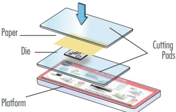
Place Sizzlits Die onto a Cutting Pad with foam side up. Place paper over the die. Place another Cutting Pad over the paper to create a "sandwich." Place "sandwich" on the platform.
